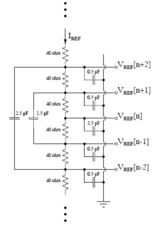
**Example: Cap stabilization 5b 1GS.s flash** Source: Esscirc 2006 Helsinki univ, Olli Viitala
