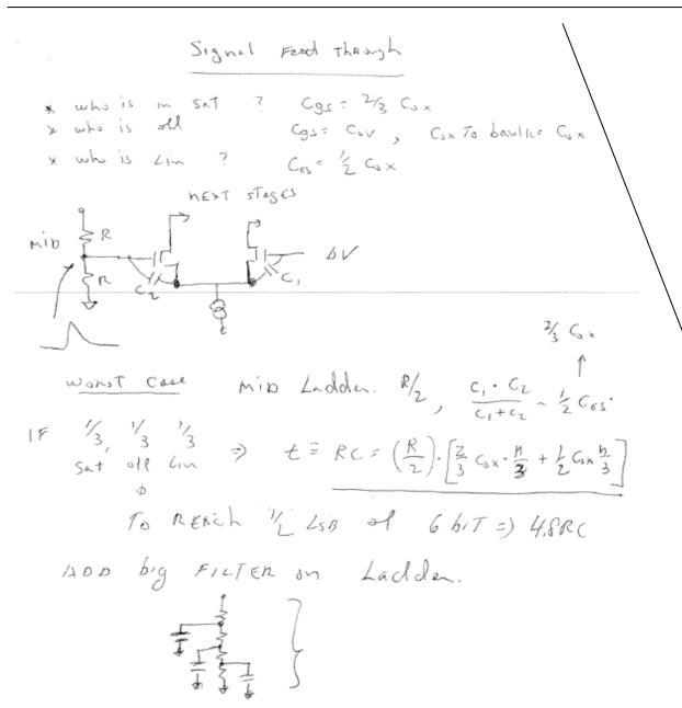
$$\frac{V_{mid}}{V_{in}} = \frac{\pi}{4} \cdot f_{in} \cdot R_{ladder} \cdot C$$
