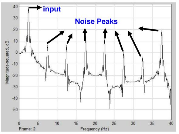
**Spectrum of a 4-channel interleaved ADC mode**
