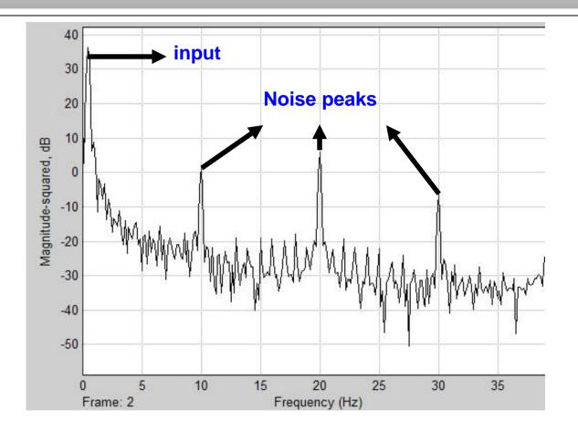
Spectrum of a 4-channel interleaved ADC model
