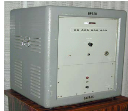
Figure 4.3: 1954 "DATRAC" 11-bit, 50-kSPS SAR ADC Designed by Bernard M. Gordon at EPSCO
