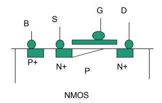
Good (for better understand) to convert the transistor to passive and active elements.
